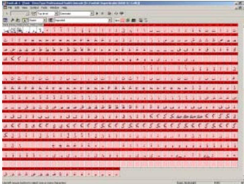
The font type used for this example (Open Type) needs internal tables for contextual glyph substitution. The new tool generates these tables dynamically.
